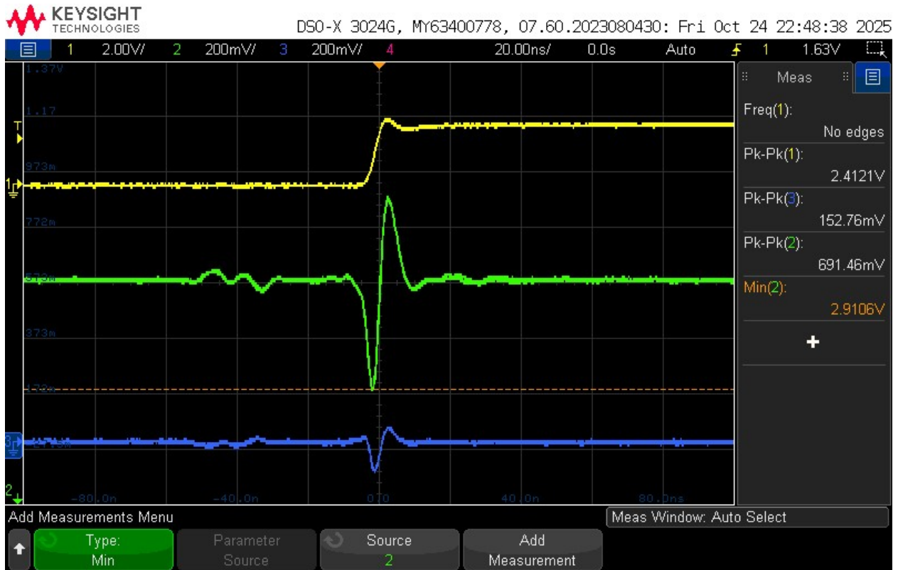
Figure 18: Oscilloscope shot of the bad hex inverter while powered by 3.3V without a decoupling capacitor on the LDO (yellow: trigger, green: quiet high, blue: quiet low).
