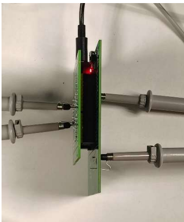
Figure 17: 5V rail collapse, "Golden" Arduino, die vs. board, test setup (yellow: D13, blue: quiet high, green: quiet low, pink: 5V rail)
