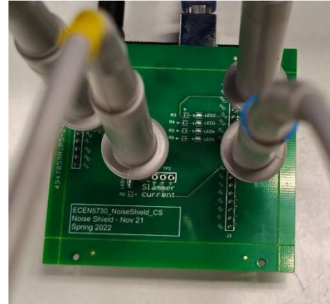
Figure 14: Slammer circuit test setup, commercial Arduino
