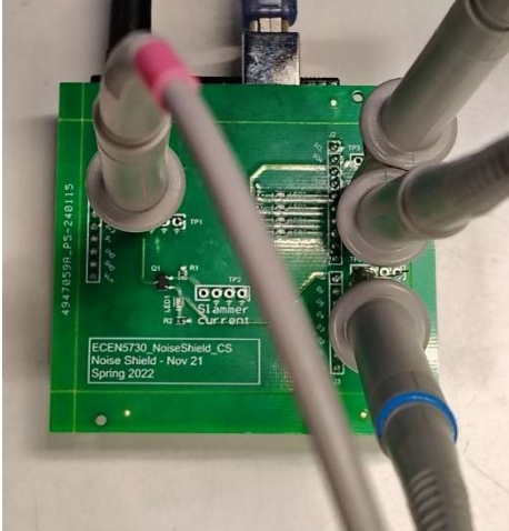
Figure 7: Switching noise test setup, "Golden" Arduino
