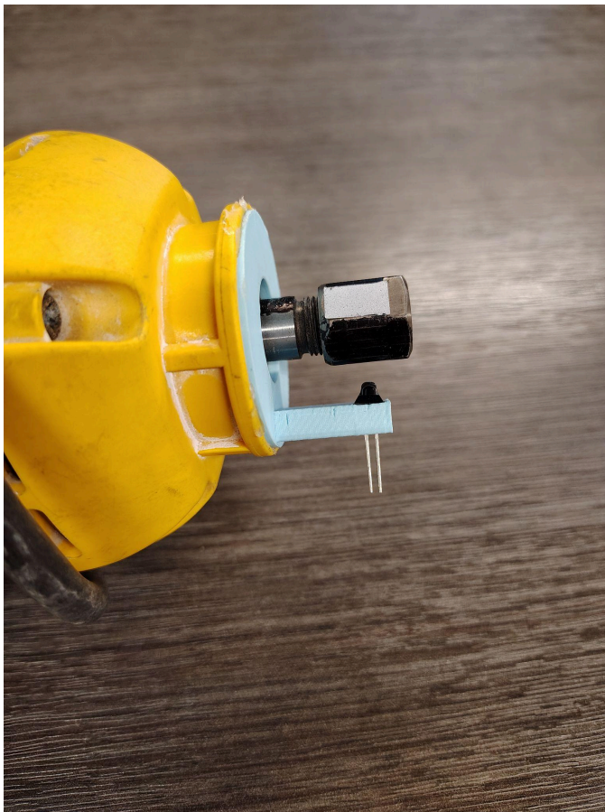
Figure 8: Emitter/detector facing dark part of collet.
