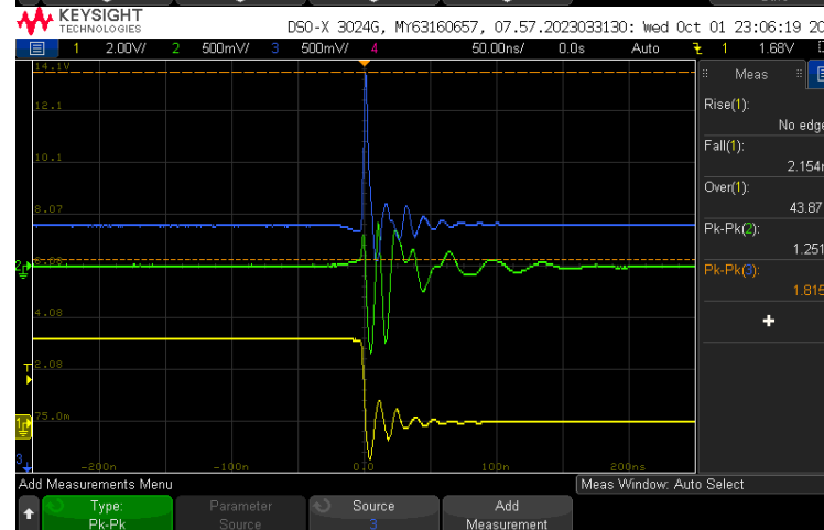
Left: Circuit w/o ground fill and far decoupling capacitor Right: Circuit w/ ground fill and far decoupling capacitor Both: Yellow = trigger, Blue = quiet high, Green = quiet low
